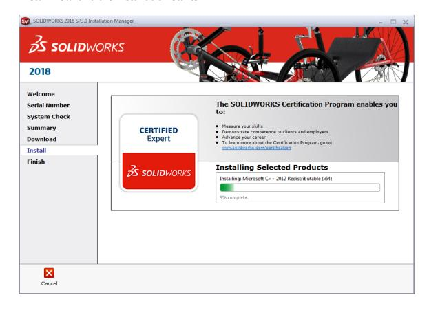
• After installation has completed, you get to decide whether to see What's New in SOLIDWORKS 2018 (select the checkbox) and you get to decide whether to be part of the SolidWorks performance feedback loop by selecting 'Yes, I want to join'. Select 'Finish'.
