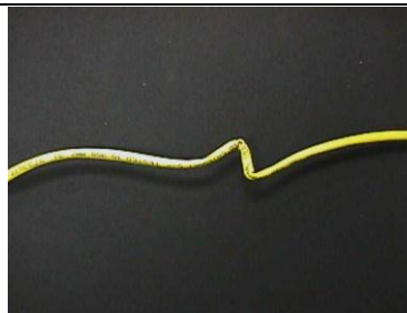
Photo 9: A cable that has been bent back upon itself.
