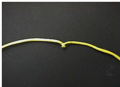
Photo 10: Another example of a loop in the cable that has been forced straight, causing severe cable trauma
